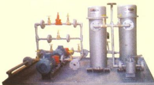
PUMPING HEATING & FILTERING UNIT
